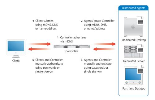
The primary components of a computational grid perform these functions:
