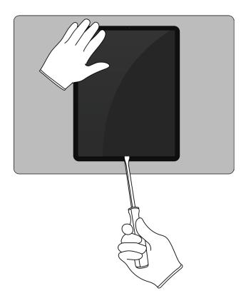
>> Remove the display by hand. Set the enclosure aside.
