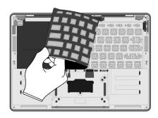
>> Separate the keyboard and the trackpad enclosure by snapping the top case in half.
