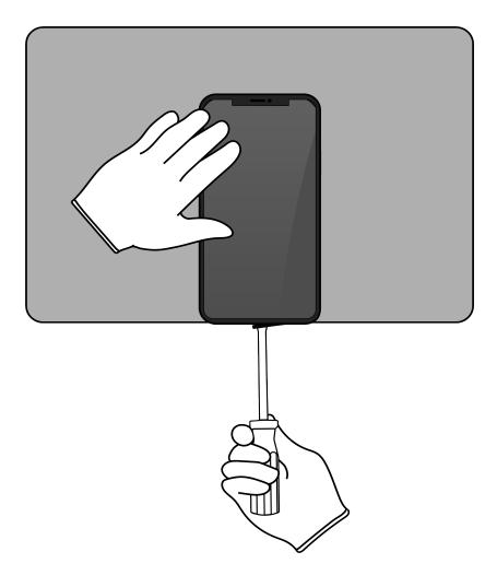
>> Remove the display by hand. Set the enclosure aside.
