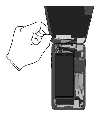
**3.** Pull the ribbon cables off the display.
