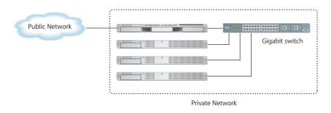
The Built-in Ethernet 1 port connects the head node to the private network and the Built-in Ethernet 2 port connects the head node to the public network.
