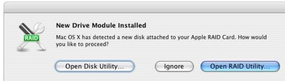
*Open Disk Utility:* Opens Disk Utility so you can erase or partition the drive and then use it in the Finder like any other disk. The resulting JBOD disk can also be read on a computer that doesn't have a RAID card installed.
