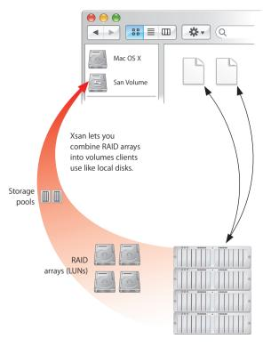
File data moves over Fibre Channel
